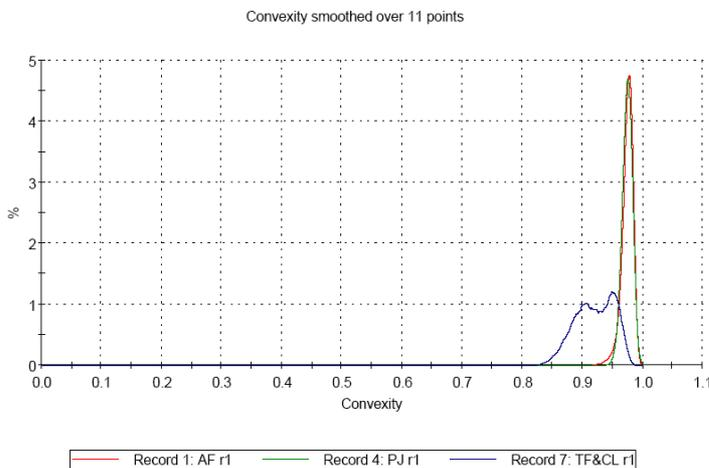
Figure 5: Convexity distribution for the three samples.
