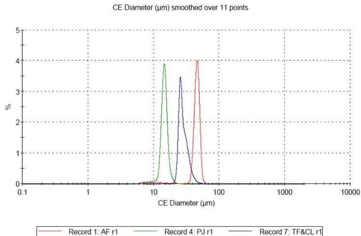
**Figure 3a:** CE diameter distribution for the three pollen samples on a number basis.
