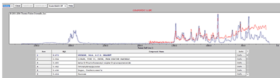
Figure 5: Result of an Advanced Spectrum Search for components 1, 2 and 11 respectively using Thermo Scientific's online database 'firsearch.com.'
