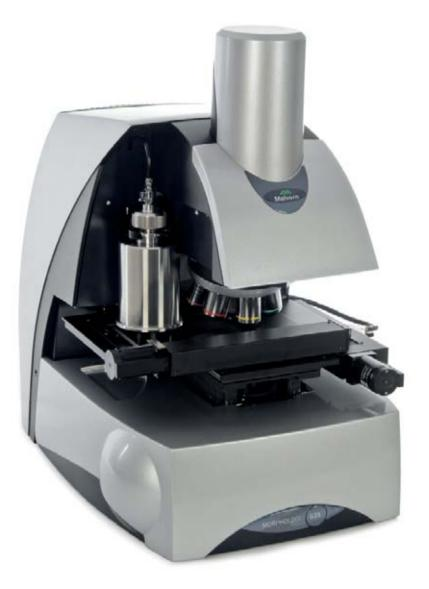
The Morphologi G3 measures the particle size and shape of dry powders, wet suspensions and particulates on filter membranes using the technique of automated static image analysis. The instrument is designed with the diverse needs of a multidisciplinary R&D lab in mind, while automation of analysis using SOPs makes it the ideal replacement for costly and timeconsuming manual microscopy measurements.
