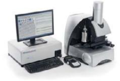
The Morphologi G3-ID brings a significant additional capability to the Morphologi range of instruments – the ability to provide chemical identification of individual particles using Raman spectroscopy. PARTICLE SIZE
