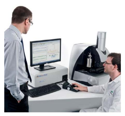
The Morphologi G3-ID provides a unique capability, combining automated static imaging features of the Morphologi G3 with chemical identification of individual particles using Raman spectroscopy. This fully automated instrument is designed to allow both particle characterization scientists with limited spectroscopy experience and more experienced spectroscopists to get an in-depth understanding of their particulate samples.
