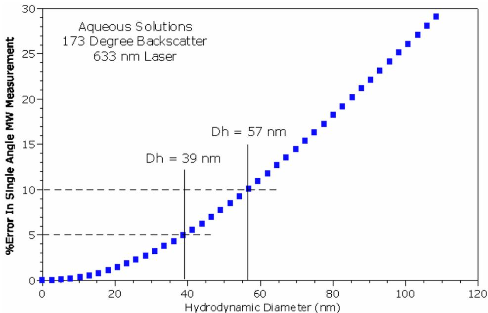
**Figure 3:** The %Error in single angle molecular weight measurements as a function of the hydrodynamic diameter for aqueous globular protein samples measured with a Zetasizer Nano ZS system.
