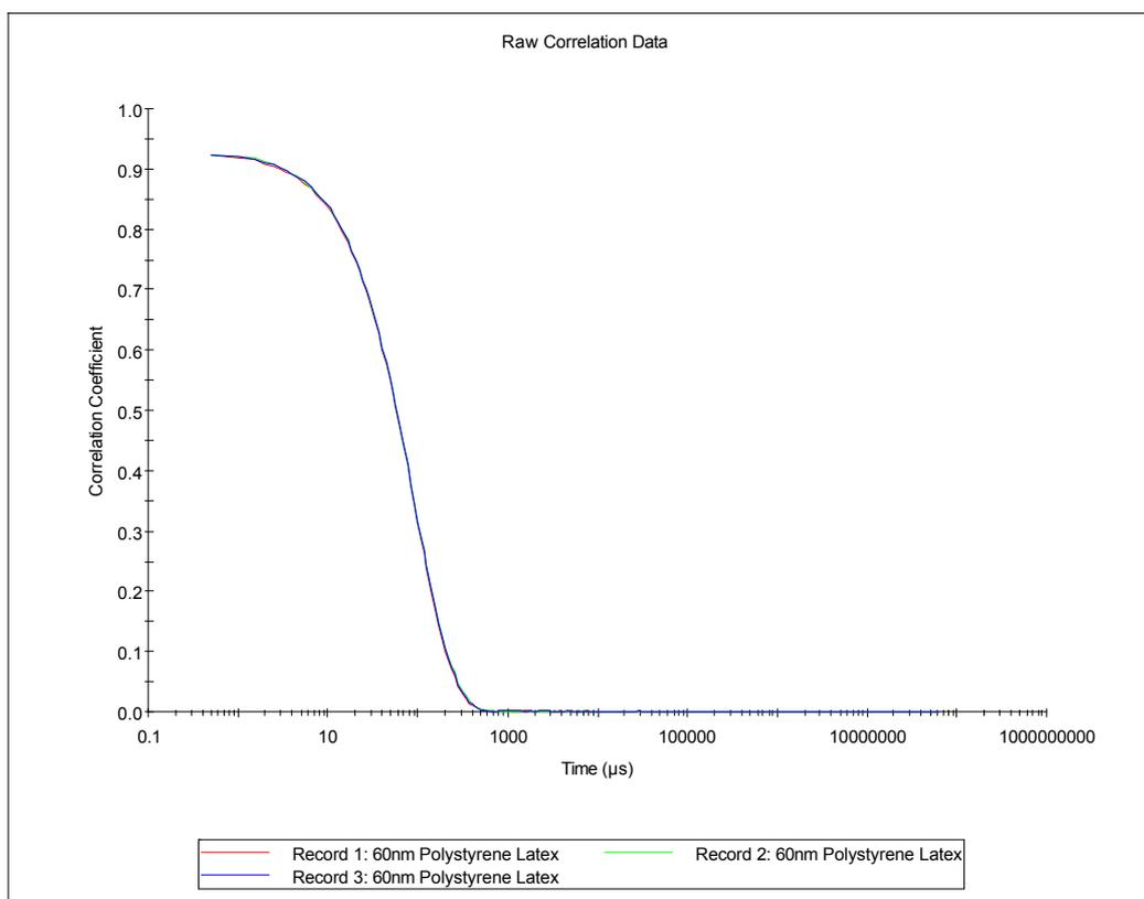
**Figure 1: 3 overlaid correlation functions from 60 nm latex with an intercept >0.9.**
