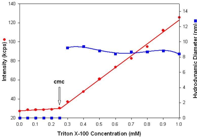
**Figure 3:** A plot of the intensity of scattered light (in kilo counts per second) and hydrodynamic diameter (in nanometres) obtained for various concentrations of triton X-100 prepared in deionised water. The intersection of the two lines at 0.25mM in the intensity data corresponds to the critical micelle concentration.
