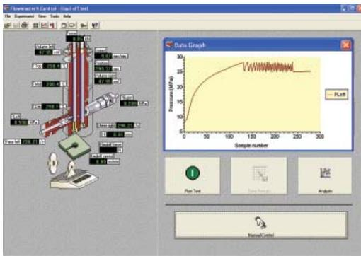
**Melt fracture/flow instability** Accelerated shear rate ramp with continuous monitoring of the pressure to detect flow instabilities, such as melt fracture which may occur during flow through a capillary die.
