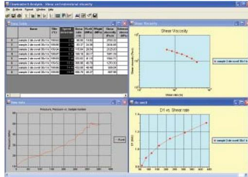
**Die swell** Measurement of the extrudate diameter close to the die exit. Directly interfaced with the control software and die swell is stored as part of the measurement data file.
