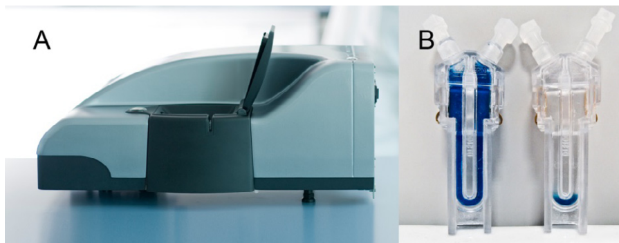
Figure 1: A: Zetasizer Nano ZSP; B: Cell entirely filled with blue dextran in 10 mM NaCl and cell filled with 10 mM NaCl loaded with 50 µl blue dextran to demonstrate the diffusion barrier technique.
