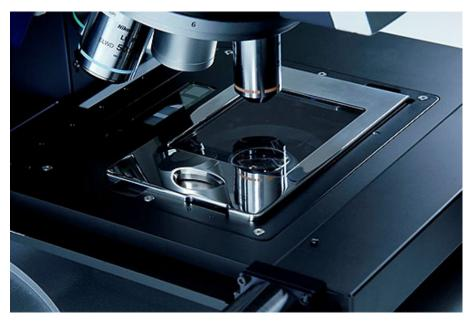
Figure 1: the Morphologi G3 wet cell
