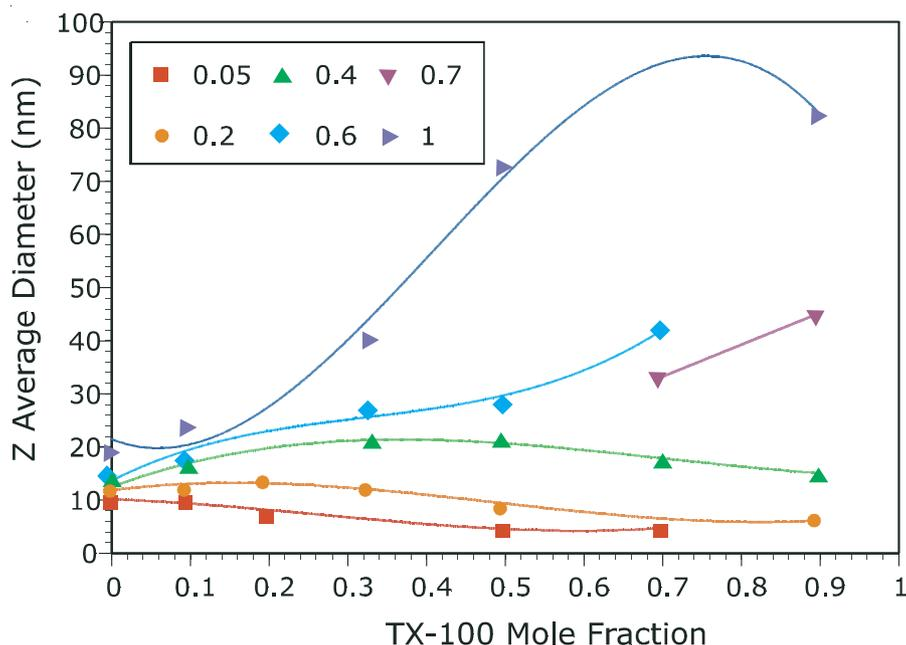
**Figure 2:** Reference data from previous experiments on the ionic strength mole fraction dependence of the size of TX-100/SDS mixed micelles.
