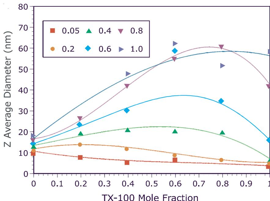
Figure 1: Comparison of the Z average diameter for TX-100/SDS mixed micelles at different ionic strengths.
