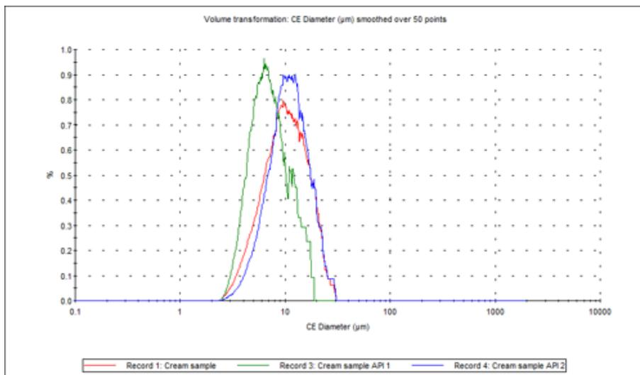
Figure 3: PSD by volume of the two actives and the blend.
