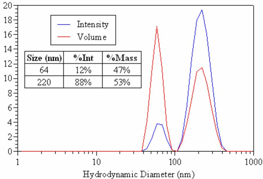
**Figure 3:** Comparison of the DLS derived intensity and volume distributions for an equal mass mixture of 62 and 220 nm latex spheres, along with the %composition results.
