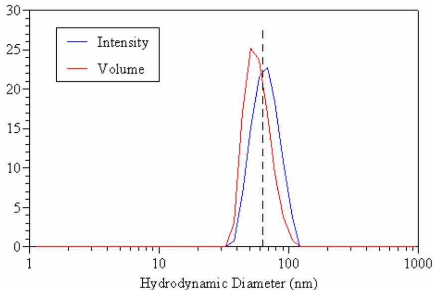
**Figure 2:** Comparison of the DLS intensity and volume distributions for a latex standard with a 62 nm hydrodynamic diameter.
