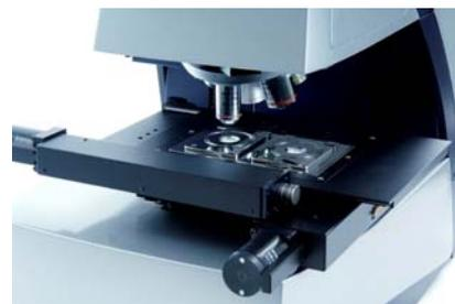
**Figure 2:** Morphologi G3 instrument with the 25 mm filter holder in place on the stage.
