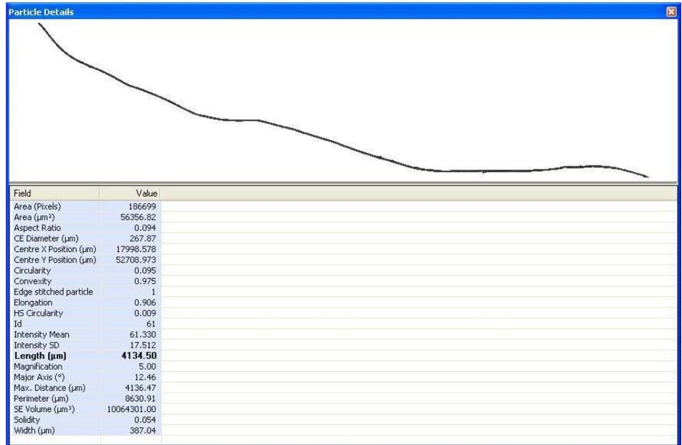
**Figure 4:** Field of view images of a particle overlapping several frames and the resulting edge stitched image with particle details. Note length of fiber is 4.1 mm.
