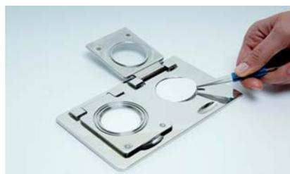
**Figure 1:** The 47 mm filter holders
