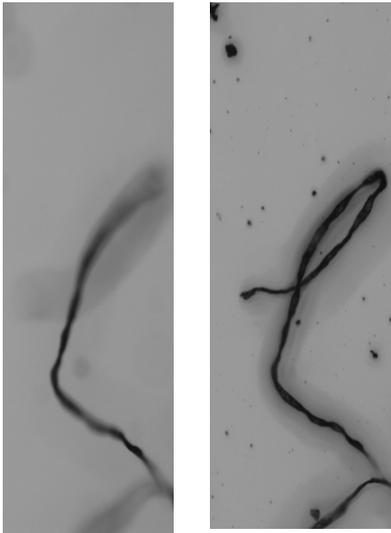
**Figure 3:** Sections of a field of view frame without (left) and with (right) z-stacking.
