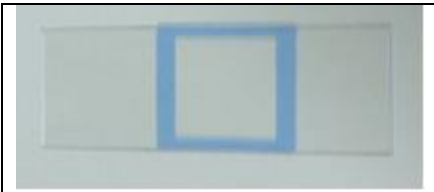
Figure 5: Slide with a gasket (sticky on both sides) placed on it. The coverslip would be placed on top.
