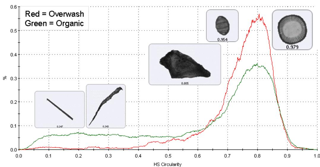
Figure 1: Particle circularity distribution of sediment samples with example particle images.
