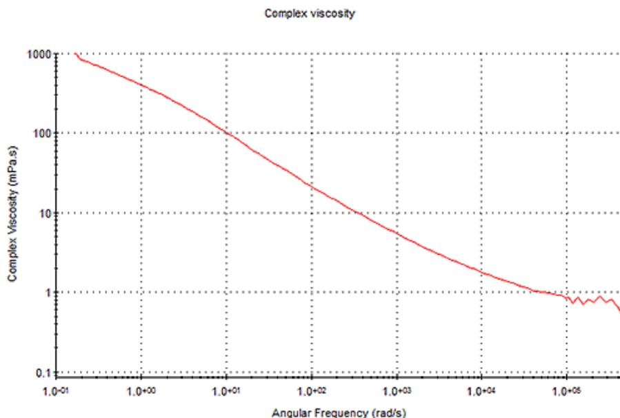
Figure 9: Complex viscosity ( $\eta^*$ ) versus frequency
