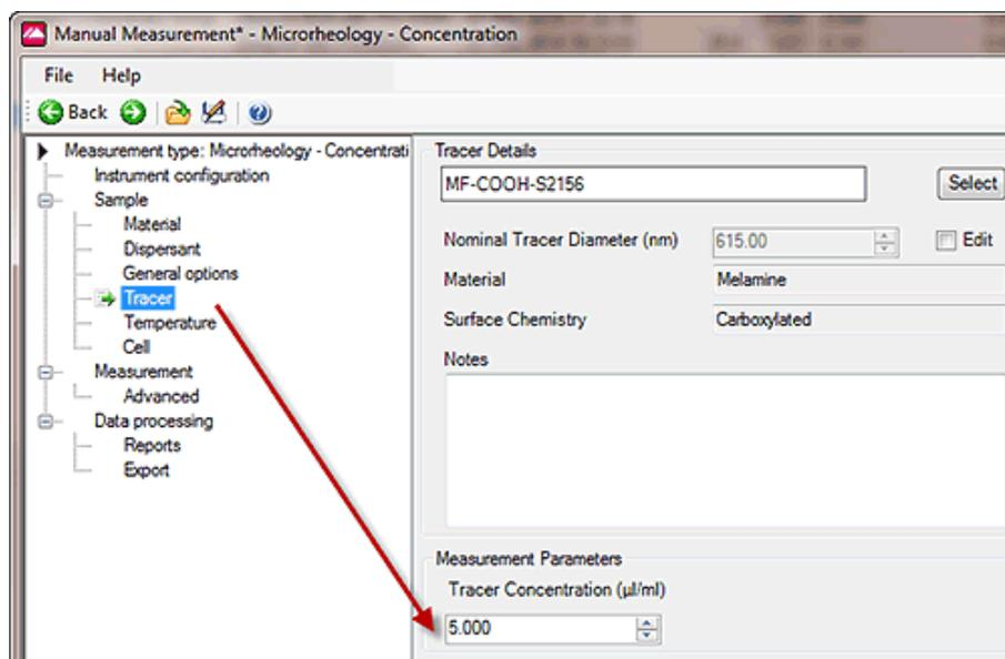
Figure 3 - Changing the tracer concentration in a concentration optimisation step
