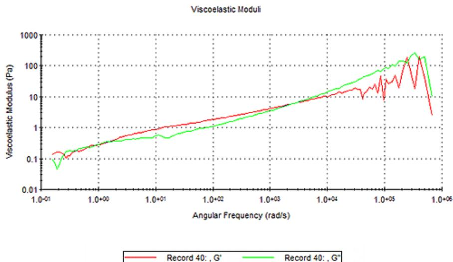
Figure 8: Viscoelastic moduli (G' and G'') versus angular frequency
