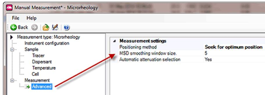
Figure 5: Applying smoothing in a microrheology measurement
