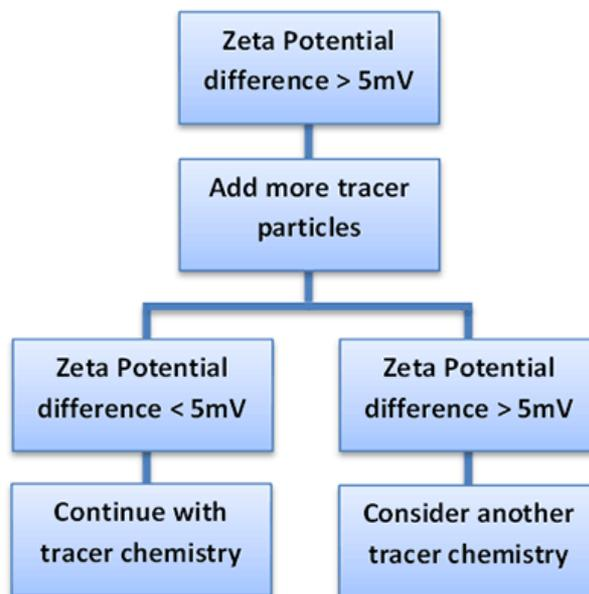
Figure 2: Decision making process for probe surface chemistry
