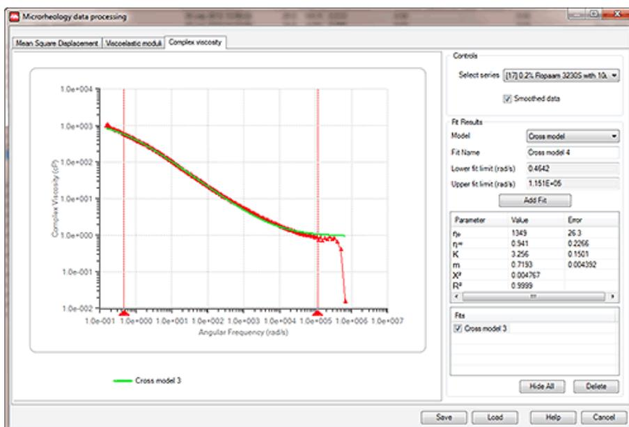
Figure 12: Model fitting using the Microrheology Utilities
