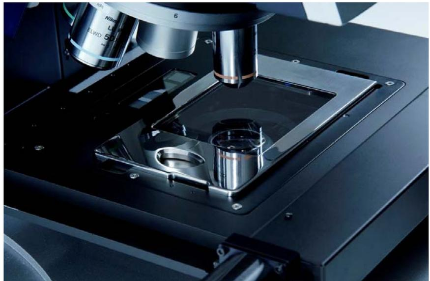
**Figure 1:** The Morphologi G3 wet cell accessory in place on the Morphologi G3 stage
