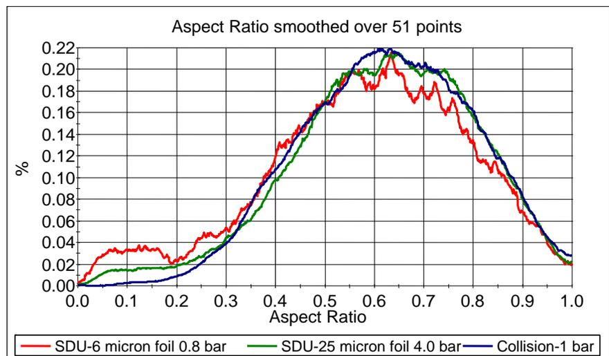
**Figure 3:** Number-weighted aspect ratio distributions for the three dispersions of a crystalline sample.
