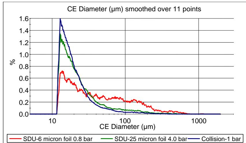
**Figure 2:** Number-weighted CE diameter distributions for three dispersions of a crystalline sample.
