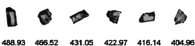
**Figure 4:** Largest six particle images from all three dispersions. The CE diameters (in  $\mu\text{m}$ ) are included below each particle image.
