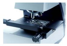
**Figure 2**: Morphologi G3 instrument with the 25 mm filter holder in place on the stage.
