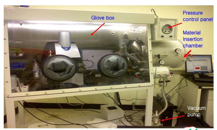
Figure 1: Morphologi G3 in the glove box system
