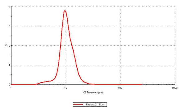
Figure 4: CE diameter distribution result for the analysis of the air sensitive Ziegler-Natta catalyst particles.
