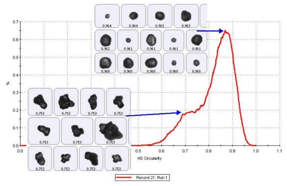
Figure 5: HS circularity distribution and images of more and less circular particles.
