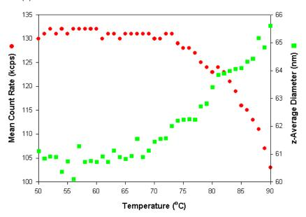
**Figure 4:** The effect of increasing temperature on the mean count rate and z-average diameter of a polymer particle dispersion.
