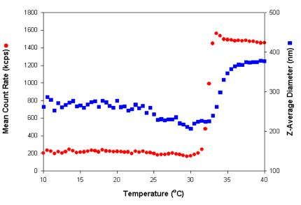
Figure 2: The mean count rate (kcps) and z-average diameter (nm) of PNIPAM plotted as a function of temperature.
