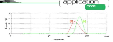
**Figure 3**: Intensity size distributions of 0.01%w/v PNIPAM measured at (a) 10°C and (b) 40°C.
