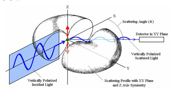
**Figure 1:** Schematic describing the absence of an angular dependence in the scattering profile for a small Rayleigh scattering particle.
