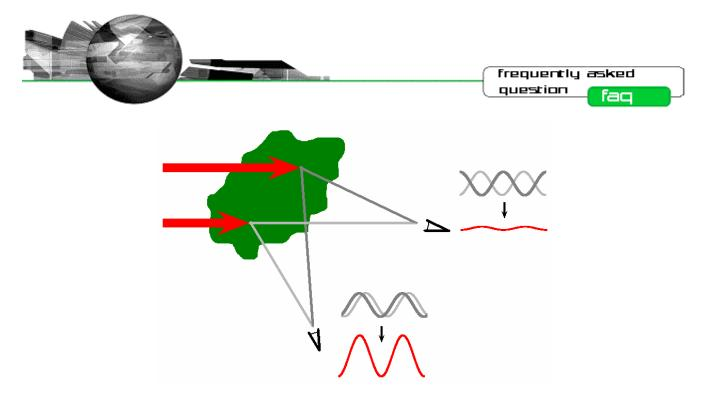
**Figure 2:** Schematic (top view) showing the constructive and destructive interference effects of multiple dipoles on the measured scattering intensity of a large particle.
