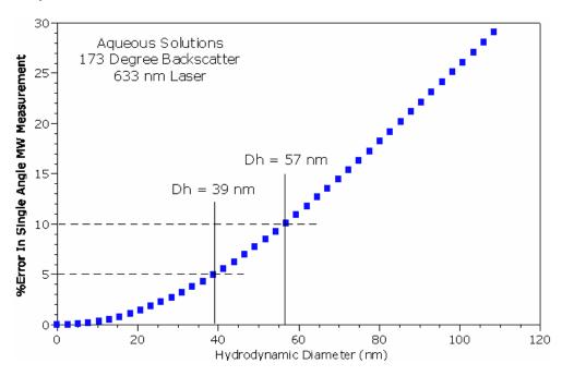
**Figure 3:** The %Error in single angle molecular weight measurements as a function of the hydrodynamic diameter for aqueous globular protein samples measured with a Zetasizer Nano ZS system.
