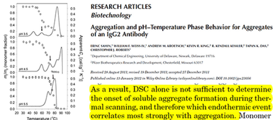
Figure 4: Paper from Sahin et al. 2012 in J. Pharm. Sci. 101, 1678-1687. The figure on the left is a representation of DSC (line, right axis) and monomer loss (circle, left axis) as functions of temperature at three pHs. The sample concentration is 1 mg/mL IgG2 samples in 10 mM citrate buffer with 1°C/min scanning rate
