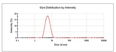
Figure 2: Intensity particle size distribution obtained for uncoated ferro oxide nanoparticles dispersed in hexane
