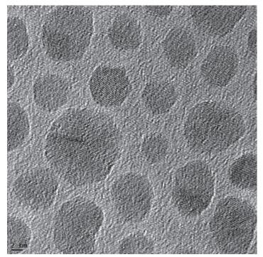
Figure 1: Transmission electron microscopy micrograph of uncoated ferric oxide nanoparticles
