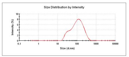
Figure 3: Intensity particle size distribution obtained for coated ferro oxide nanoparticles dispersed in hexane
