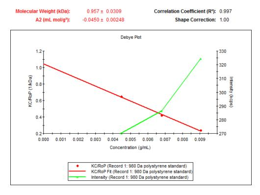
Figure 19: Verifying the minimum molecular weight for the Zetasizer  $\mu V$
