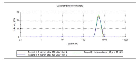
Figure 8: Verifying the maximum size on the Zetasizer  $\mu V$
