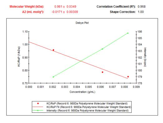
**Figure 17:** Verifying the minimum molecular weight for the Zetasizer Nano S/ZS
