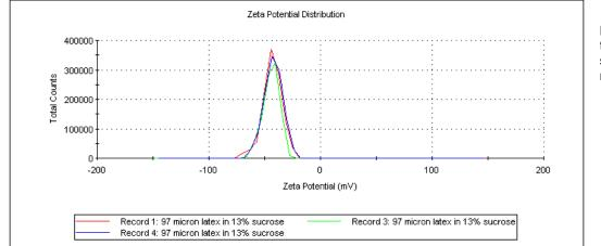
Figure 14: Verifying the maximum particle size for zeta potential measurement
