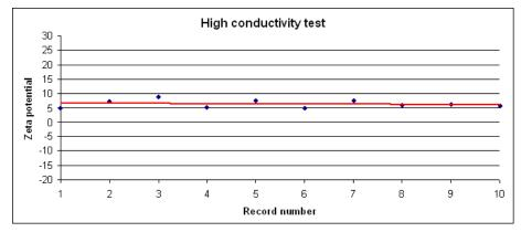
Figure 15: Verifying the maximum conductivity of 200mS/cm for zeta potential measurement
