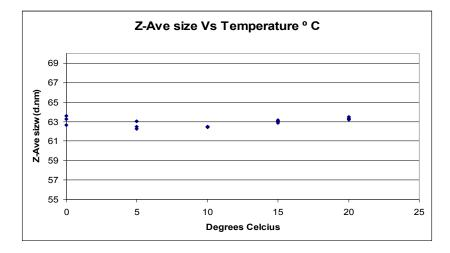
Figure 9: Verifying the temperature stability of the Zetasizer platforms
