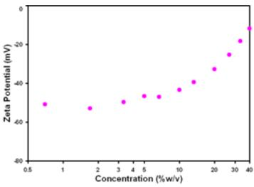
Figure 16: Verifying the maximum concentration of 40%w/v for zeta potential measurement
