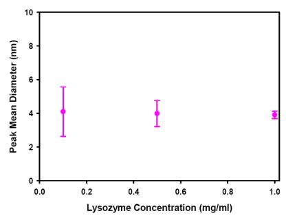
**Figure 11:** Verifying the minimum concentration range in of 0.1mg/mL lysozyme for the Zetasizer Nano S/ZS
