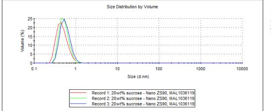
Figure 3: Verifying the minimum size on the Zetasizer Nano S90/ZS90
