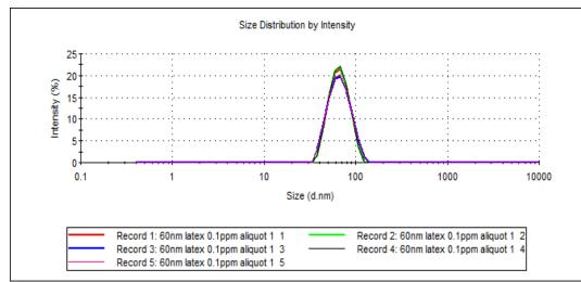
**Figure 10:** Verifying the minimum concentration range of 0.1ppm for the Zetasizer Nano S/ZS
