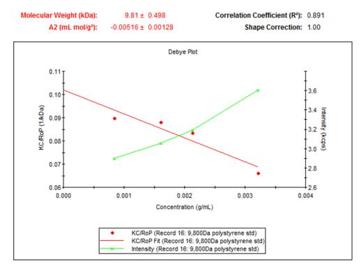
**Figure 18:** Verifying the minimum molecular weight for the Zetasizer Nano S90/ZS90
